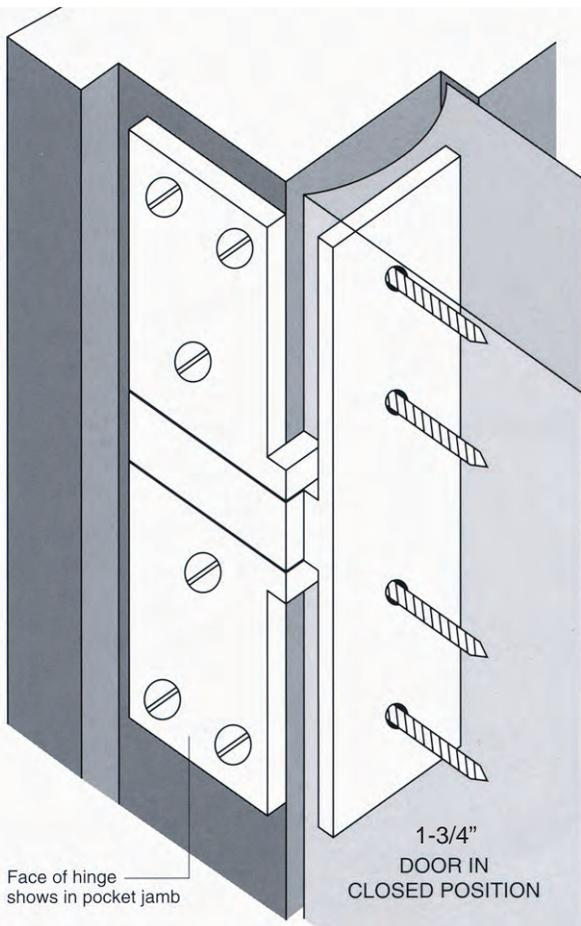
This hinge allows a door to swing clear of the opening and fold back into a pocket at right angle to the closed position. No part of the hinge projects beyond the face of the door in either opened or closed position.
